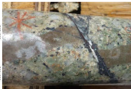
Sericite altered Bethlehem phase. Felsphic dike cut and offset by quartz-bornite veinlet.
