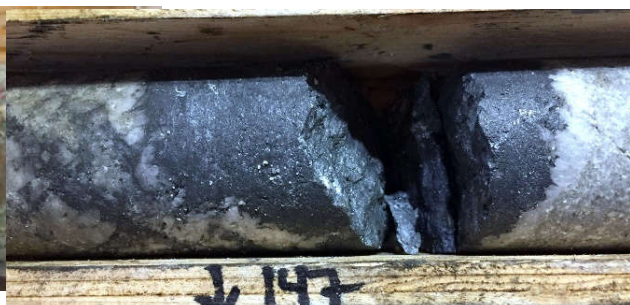
R17-02 Massive chalcocite: Portion of 5.0m 4.41% Cu, 20.0 g/t Ag, 0.21 g/t Au, 0.031% Mo, 6.86 g/t Re
