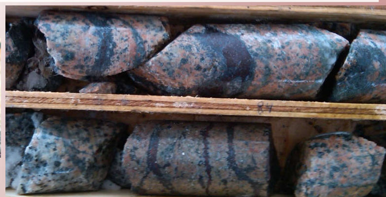
R11-36 K-spar-qtz-sericite bornite veins. Portion of 2.5m sample with 1.11% Cu, 0.46 g/t Au, 0.031% Mo, 0.80 g/t Re
