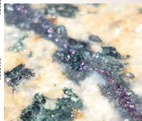
Bornite in quartz green mica, sericite-muscovite veinlet and selective replacement of chlorite altered mafics.
