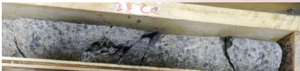
R17-05 chalcocite-bornite qtz-ser-clay Portion of 2.5m 0.89% Cu, 0.38 g/t Au, 0.003% Mo, 0.54 g/t Re
